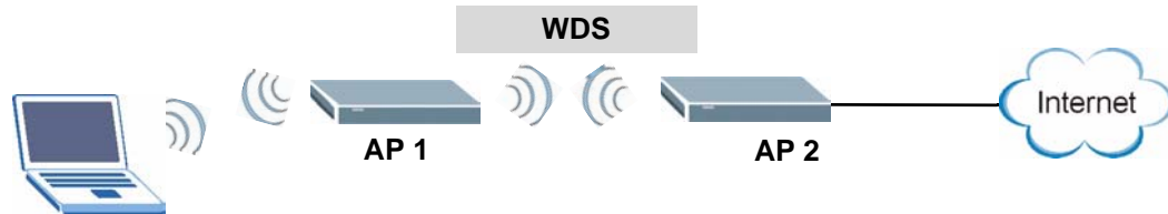
Figure 74 Wireless Bridge Example
