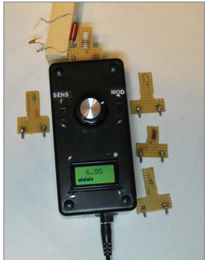
Photo 1 —This digital dip meter prototype shows an external LC circuit and the various tuning coils. The block of wood is used so the test circuit will be the same height as the dip meter coil.
