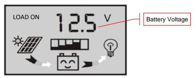
By pressing the 'DOWN / LOAD' button from this interface, you can turn the load ON or OFF. NOTE: The Load on/off function is not available in any other interface.
