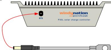
2) Secure the ring terminal on the BTS directly to any side of the battery to be monitored, below the electrolyte level as shown below. When multiple batteries are used, it is best to place the sensor between batteries and place the batteries in an insulated box to reduce the influence of the ambient temperature outside the battery enclosure.
