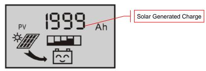
NOTE: Press the 'MODE' button for over 5 seconds to clear/reset the cumulative, generating charge (Ah).
