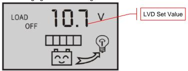
NOTE: To change the LVD voltage, press the 'MODE' button for over 5 seconds until the number starts to blink / flicker. The controller will enter the adjustable mode, where you can use the 'UP' and 'DOWN' buttons to adjust the parameter. After the value has been set, press the 'MODE' button for over 5 seconds to exit the adjustable mode and store the setting.
