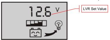
NOTE: To change the LVR voltage, press the 'MODE' button for over 5 seconds until the number starts to blink / flicker. The controller will enter the adjustable mode, where you can use the 'UP' and 'DOWN' buttons
