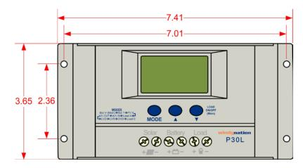
IMPORTANT: For best results, mount the charge controller and batteries as close to the panels as practical.
