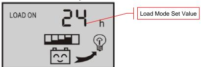
NOTE: To change the Load Control value, press the 'MODE' button for over 5 seconds until the number starts to blink / flicker. The controller will enter the adjustable mode, where you can use the 'UP' and 'DOWN' buttons to adjust the parameter. After the value has been set, press the 'MODE' button for over 5 seconds to exit the adjustable mode and store the setting.
