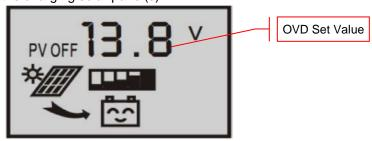
NOTE: To change the OVD value, press the 'MODE' button for over 5 seconds until the number starts to blink / flicker. The controller will enter the adjustable mode, where you can use the 'UP' and 'DOWN' buttons to adjust the parameter. After the value has been set, press the 'MODE' button for over 5 seconds to exit the adjustable mode and store the setting.
