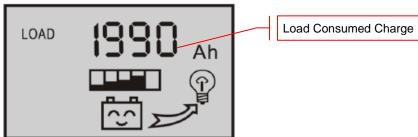
NOTE: Press the 'MODE' button for over 5 seconds to clear/reset the cumulative, consumed charge (Ah).
