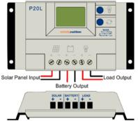
**IMPORTANT:** The screw-down terminals on the charge controller accept 8~26AWG wire.
