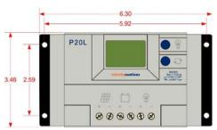
IMPORTANT: For best results, mount the charge controller and batteries as close to the panels as practical.
