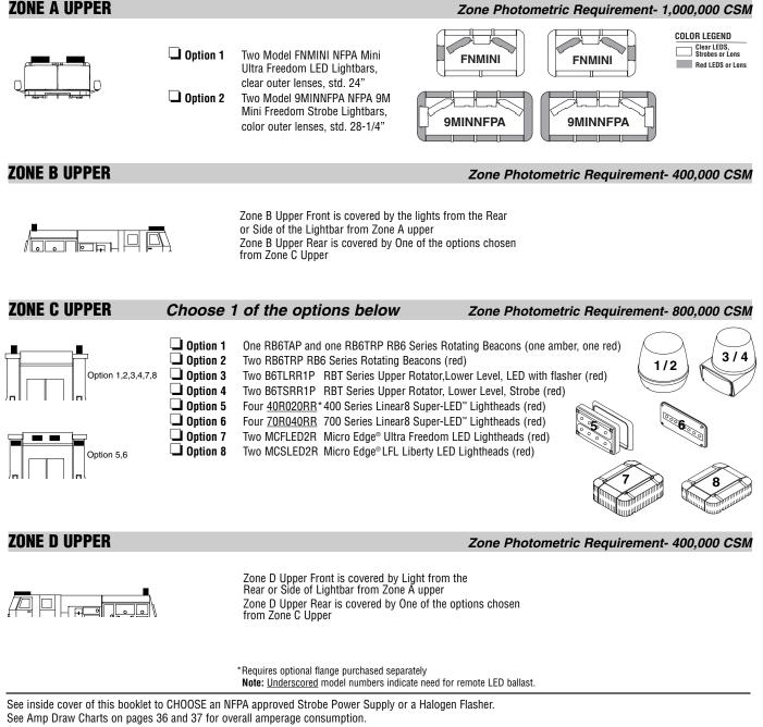
Some LED lightheads have internal flasher module and do not need a flasher unless a specific flash sequence is needed. <u>Underscored</u> LED lightheads need a remote ballast to operate.
