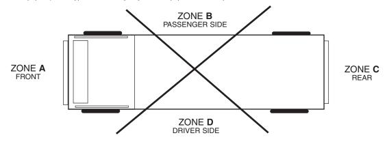
**Large apparatus** is defined as an apparatus that has a bumper to bumper length of 22 feet or greater. On large apparatus, the minimum optical warning system will draw no more than an average of 45 amps total for all upper & lower level warning lights combined. There may be the need to exceed the over all average amperage draw of 45 amps when additional lower zone mid-ship lights are needed.
