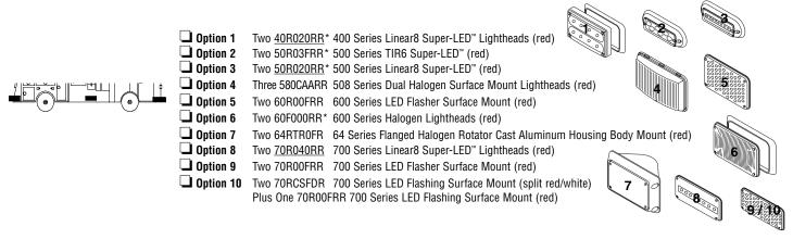
Note: Choosing one of the options listed in each zone is the minimum zone requirement that is needed to meet the NFPA 1901 Standard for Automotive Fire Apparatus 1999 Edition, Table 11-8 12.4 (Minimum Optical Power Requirements for Apparatus). If additional lighting is needed to meet lower zone distance requirements only, you can use any of our warning lightheads shown on pages 33, 34 or 35 of this brochure.
