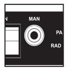
MAN BUTTON - The Manual button generates a variety of tones, depending on what position the rotary knob is in. For further explanation of this button's function, refer to Rotary Switch Operations.
