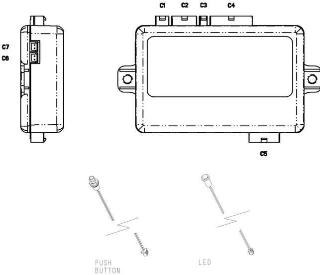
1. Plug the LED into C6 and the push button into C7 on the receiver. Your OEM may have already installed these in your vehicle.
