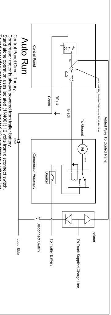
Towed operation uses isolated (battery isolator) 12 volts from truck charge line directly connected to pressure switch.
