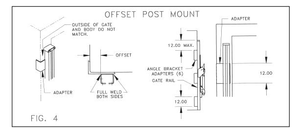
**Step 5** If the truck's rear corner posts are aluminum, six steel angle brackets .25" minimum wall thickness x 12" must be fabricated and attached as shown in figure 5. Bolt brackets to rear of vehicle as required to support the load.
