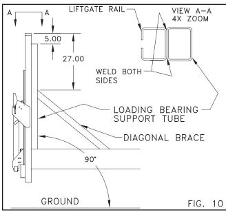
**Step 10** If liftgate installation is on a flatbed vehicle, fabricate load bearing support tubes and diagonal braces as shown in Figure 10. Square the support tubes with the bed and perpendicular to the ground as shown, and weld braces to vehicle body and support tubes. Then weld liftgate rails to support tubes on both the inside and outside corners of each rail.
