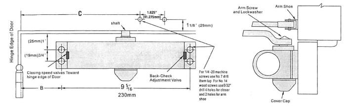
RIGHT HAND DOOR ILLUSTRATED Same dimensions apply for left Hand Door measured from the hinge edge.
