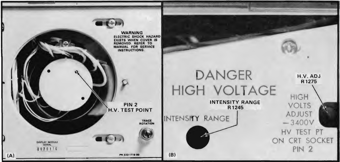
Fig. 7-2. Location of (A) CRT socket access and (B) R1275, H V Adj R1245, Intensity Range.
