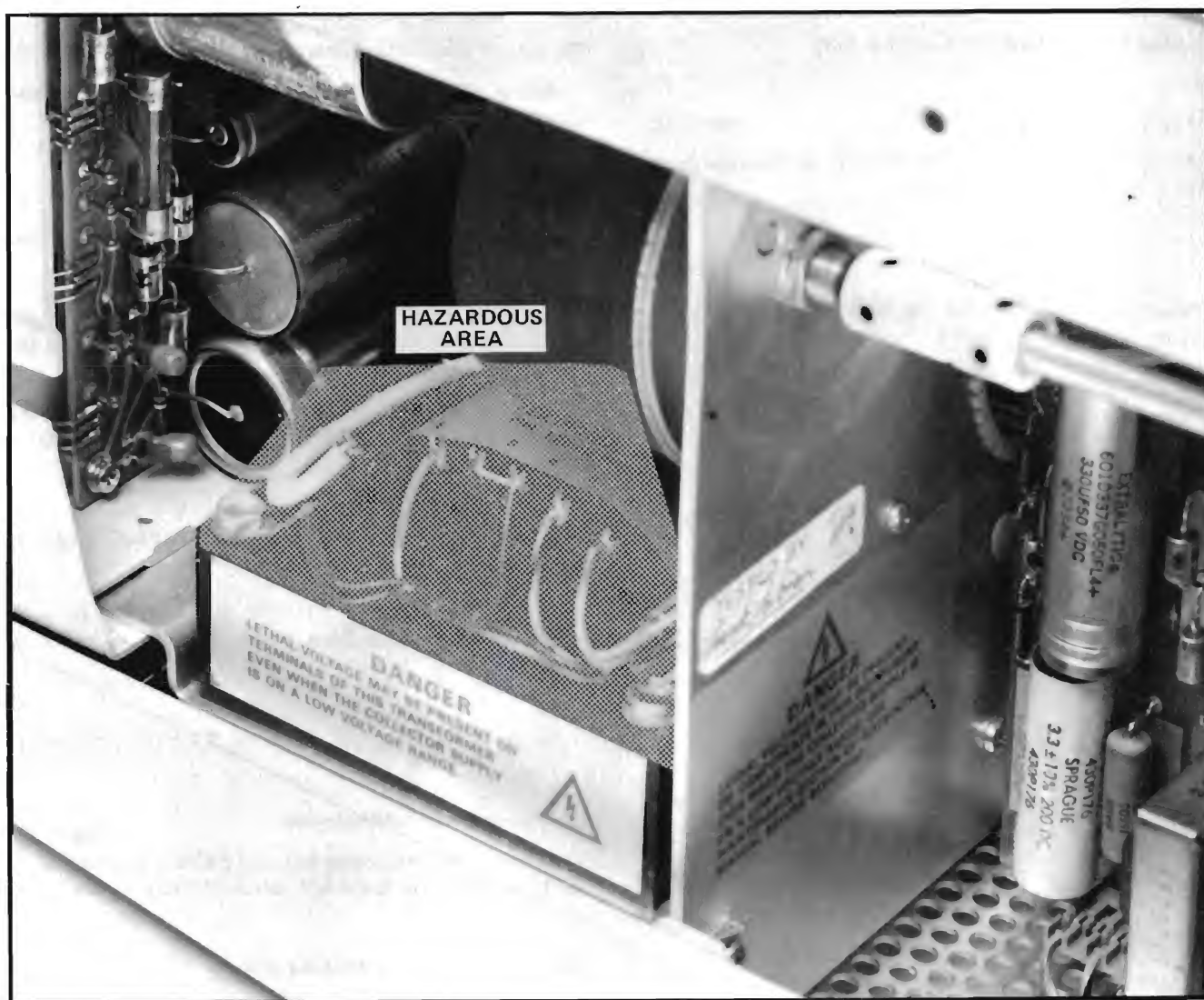
Fig. 5-12. Location of the danger areas adjacent to the Power Supply test points.
