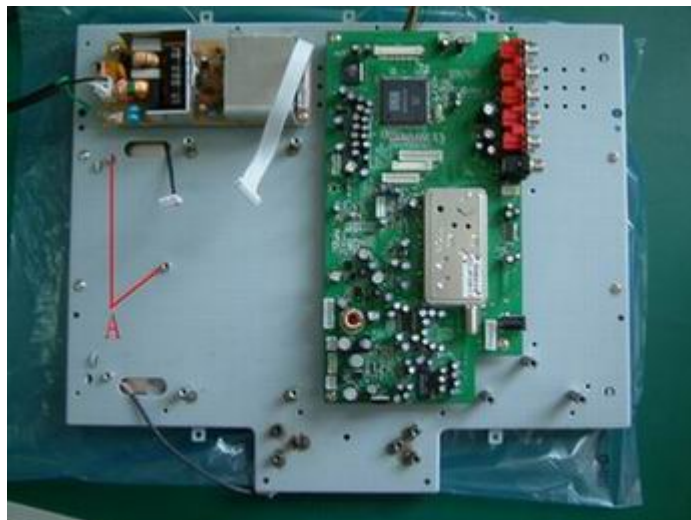
10. Fig10: Remove the HI-voltage Board and the screws for its fixing from(A) positions and remove the base.
