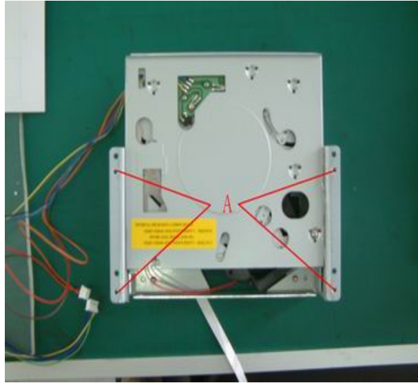
9. Fig9: Remove the front panel and the screws for its fixing from (A) positions.
