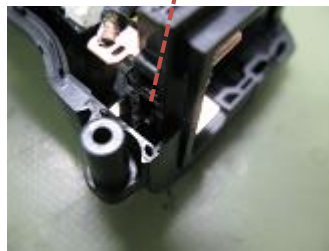
Battery terminal is set correctly
