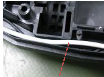
Wire harnesses are set correctly
