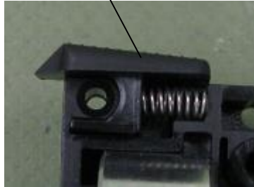
Collector Lock with spring
