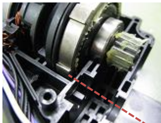
Ring Gear is fitted correctly
