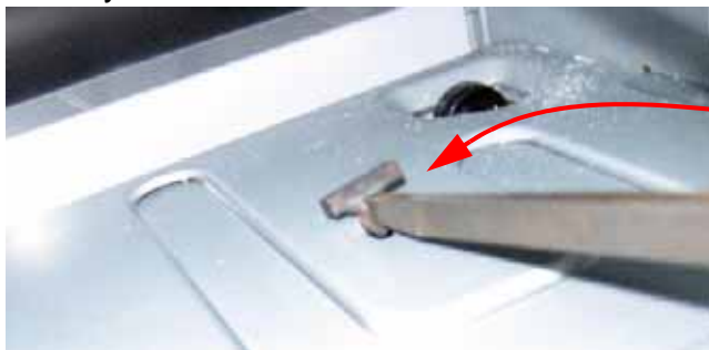
Special Belt Fitting Tool Part No. C00142716
