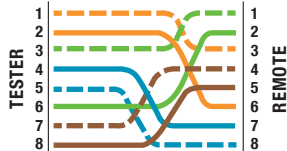
T568B Cross Over Data Cable Properly Wired
