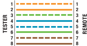
T568B Cross Over Data Cable Properly Wired
