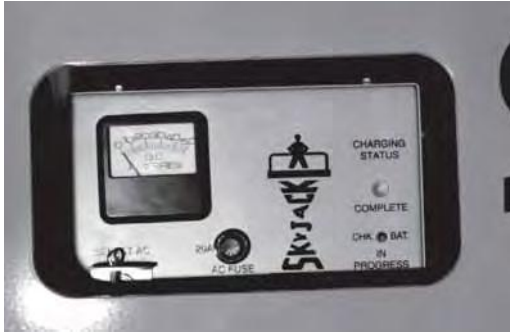
Figure 2-15. Bycan Automatic Battery Charger
