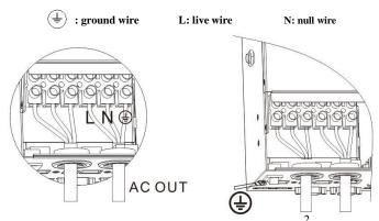
Note: use thick ground cable as far as possible (with cable section not less than 4mm<sup>2</sup>), place the ground point to be close to the all-in-one machine as far as possible and choose shorter ground wire to the greatest extent
