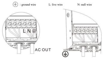
Note: use thick ground cable as far as possible (with cable section not less than 4mm2), place the ground point to be close to the all-in-one machine as far as possible and choose shorter ground wire to the greatest extent
