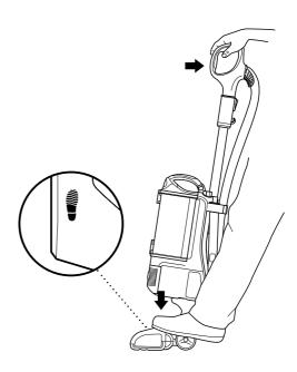
Plug power cord into outlet. Place foot on floor nozzle and tilt handle back.
