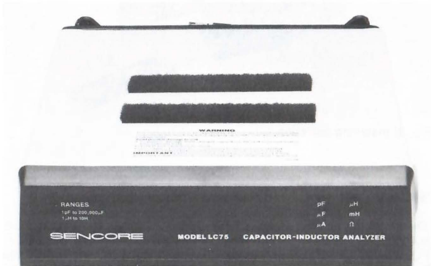
Fig. 2: Velcro® strips installed on the top of a “Z METER”.
