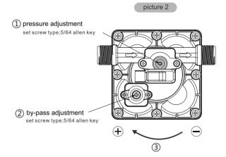
\*Remove the pressure adjustment screw completely, mark the screw in relation to the switch housing for reference as to number of "turns", start screwing the set screw clockwise "9 to 9-1/2 turns", as the ③. This will increase the pressure to shut-off at approximately 60 psi.
