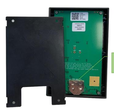
Slide the battery up to remove.
