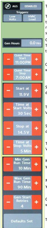
Tap to Enable/Disable AGS. A Warning screen will require action to enable.
