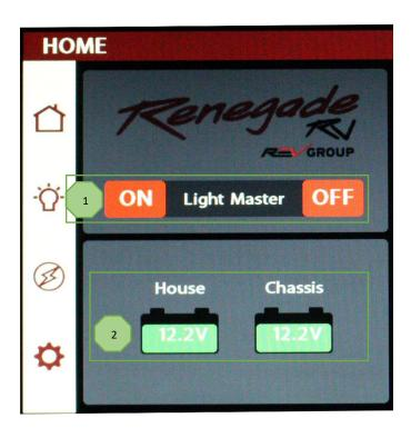
Battery Level Indicators - These graphics will indicate the battery voltage for the House and Chassis batteries. The graphics will display Green while above 12V and Red while below 12V.
