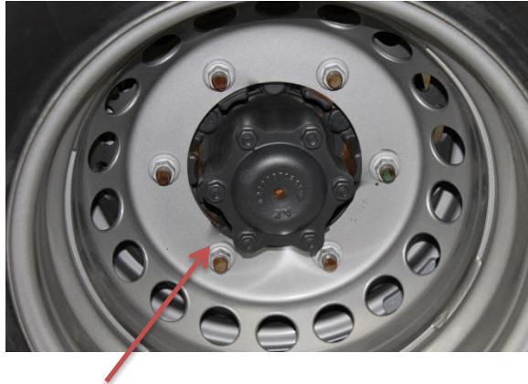
Steel Wheel Lug Nut and Washer ( Hex Flange Nut with Split Cone Washer)
