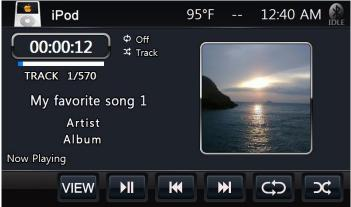
The Infotainment Center can also be connected to your Apple iPod or iPhone. When the iPod is connected, press the **iPod** icon in the Main Menu. The iPod mode can be left any time by pressing the iPod icon at the top left of the screen. To access and use the iPod feature please connect your iPod/iPhone device first to the iPod cable provided.
