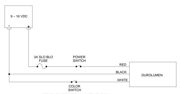
COLOR SWITCH OPEN = WHITE LED'S ON COLOR SWITCH CLOSED = RED LED'S ON
