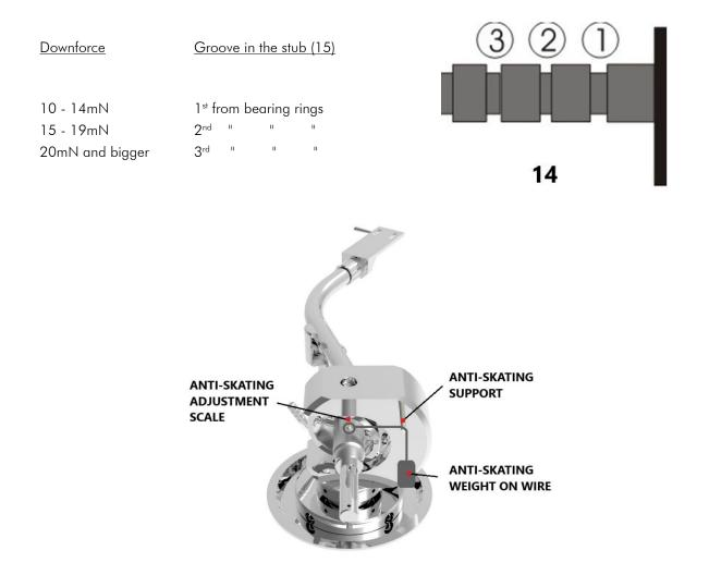
Hang the loop of the thread of the anti-skating weight in the groove of the anti-skating scale (14) corresponding to the downforce applied to your cartridge and hang the thread in the groove of the wire support (15).
