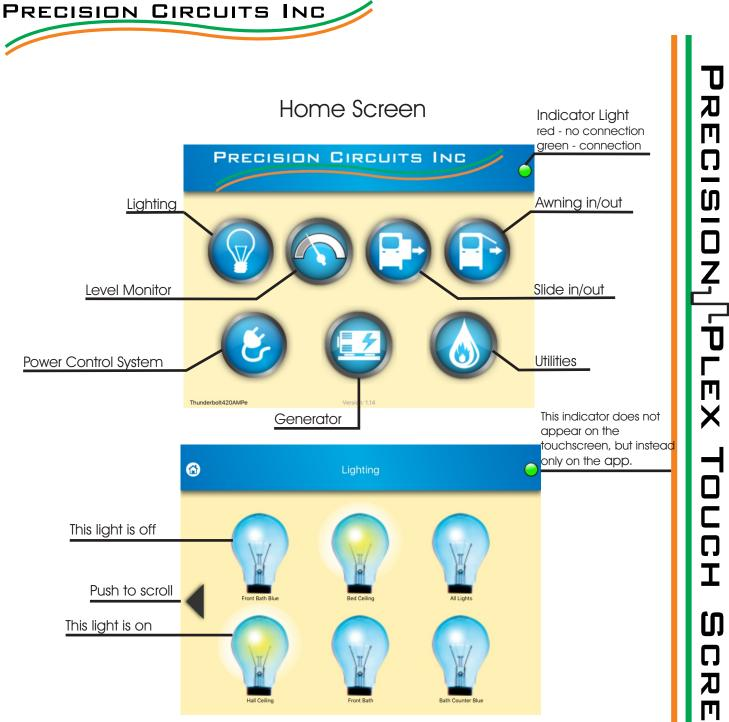
Lighting - Control every light in your RV from this screen. Use the arrow keys to scroll left and right to view each lighting option. In the image above, "Hall Ceiling" and "Bed Ceiling" indicate a light is on.
