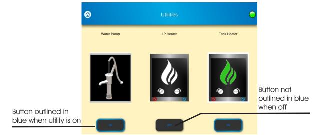
Utilities: This screen allows the user to turn on or off the water pump, liquid propane heater, and tank heater as necessary or as situations demand. Simply touch the button underneath the image to turn on or off. On the touch screen touching the on/off button or the image will operate the feature.
