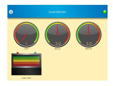
Level Monitoring: On this screen, one can monitor the levels of fresh water, grey water, black water, and battery charge. Notice the difference in how the colors red and green appear on Fresh as compared to Grey and Black. When the dial points in the red section of the gauge the level is critical, whereas pointing in the green section indicates good levels. Likewise, when the battery has green it is in a good state and when it has only red it has a low charge.
