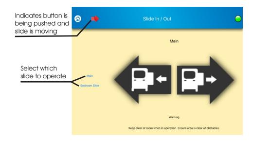
Slide IN/OUT: To move slide out, check the area surrounding your RV, and if there is enough room, push and hold the button on the right. Letting go of the button will stop the slide from moving. To bring the slide back in, push and hold the button on the left. If more than one person is trying to operate the slide via multiple devices, the person who was first in attempting operation will be the one able to carry out execution.
