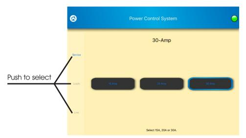
Power Control System: When the user to plugs in to anything less than 30 Amps, the corresponding service must be selected from the Power Control System screen. This is done simply by pushing the desired power amount. Failure to chose the correct service may cause a circuit breaker to be tripped.
