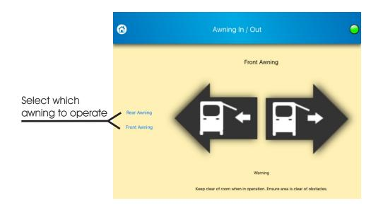
**Awning IN/OUT:** To move awning out, check the area surrounding your RV, and if there is enough room, push and hold the button on the right. Letting go of the button will stop the awning from moving. To bring the awning back in, push and hold the button on the left. If more than one person is trying to operate the awning via multiple devices, the person who was first in attempting operation will be the one able to carry out execution.
