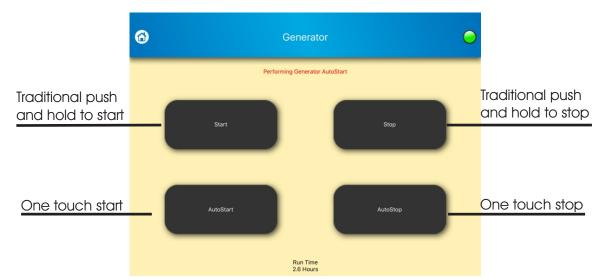
Generator: The Start and Stop buttons run the generator and stop the generator in the fashion that experienced RV users are accustomed to; the user must hold the Start button until the generator turns on and remains on. Likewise the Stop button must be pushed and held until the generator turns completely off, simply pushing the button may not stop the generator.
