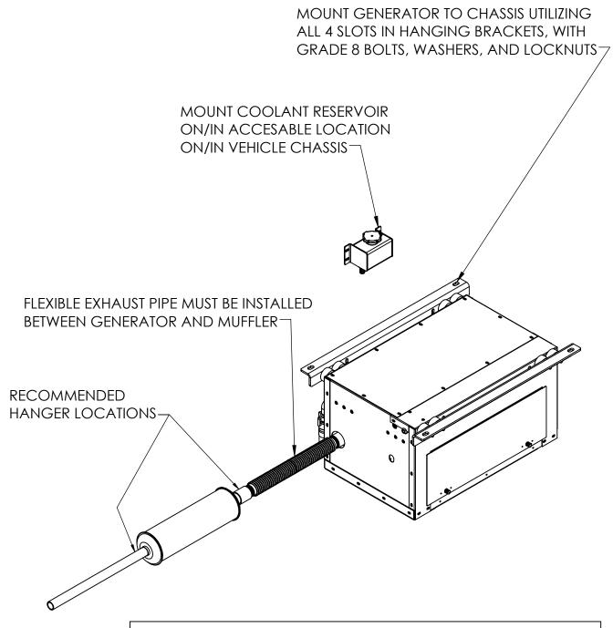
MUFFLER AND FLEX PIPE MUST BE SUPPORTED IN AT LEAST 2 LOCATIONS WITH EXHAUST HANGERS MOUNTED BETWEEN THE CHASSIS AND MUFFLER. IN CERTAIN APPLICATIONS THE FLEX PIPE MUST ALSO BE SUPPORTED WITH EXHAUST HANGERS
