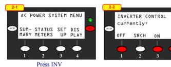
Press OFF / ON to turn inverter off or on. Then OK to go back to AC Power Systems Menu. A good way to do a quick inverter reset is turn OFF for 5 seconds then ON again. Also, unplugging the Cat 5 from the Mate is a good remote reset.
