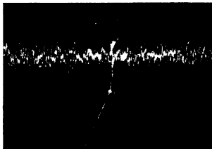
TP FO (Focus out) Vertical : 0.5V/div. Horizontal : 0.5 ms/div. DC, Ground: Center
