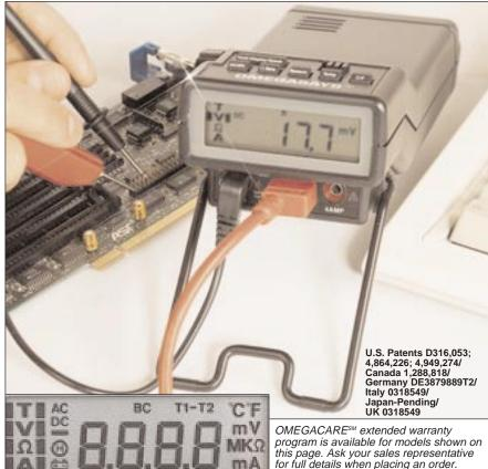
input (T1, T2 or T1-T2), display hold and low battery. All DMM connections plug into the front of the unit. Thermocouples, earphones and the ac adaptor plug into the rear panel of the unit, which also contains a three-position volume selector switch.
