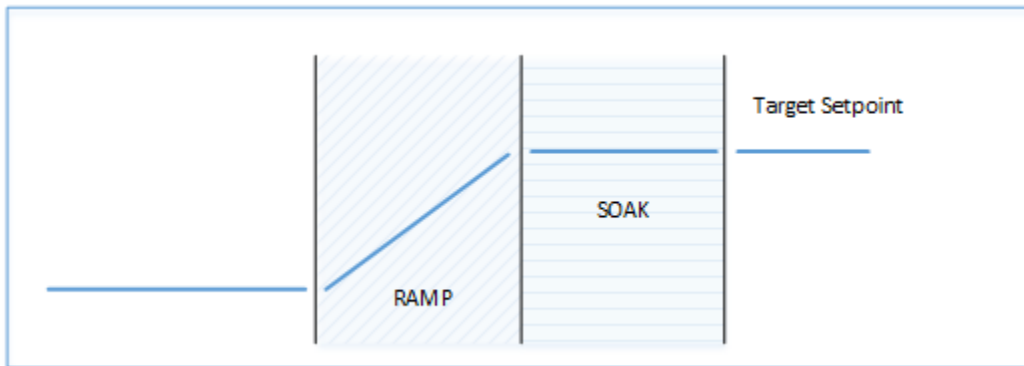
Figure 14. Ramp & Soak Process Variable Period of Time.
