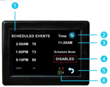
Set points may be changed on a time-based schedule. The mode used will be the heating or cooling mode set on the main screen.
