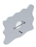
**Step 2:** Screw in one screw and level the buttons so the display will be straight when installed.
