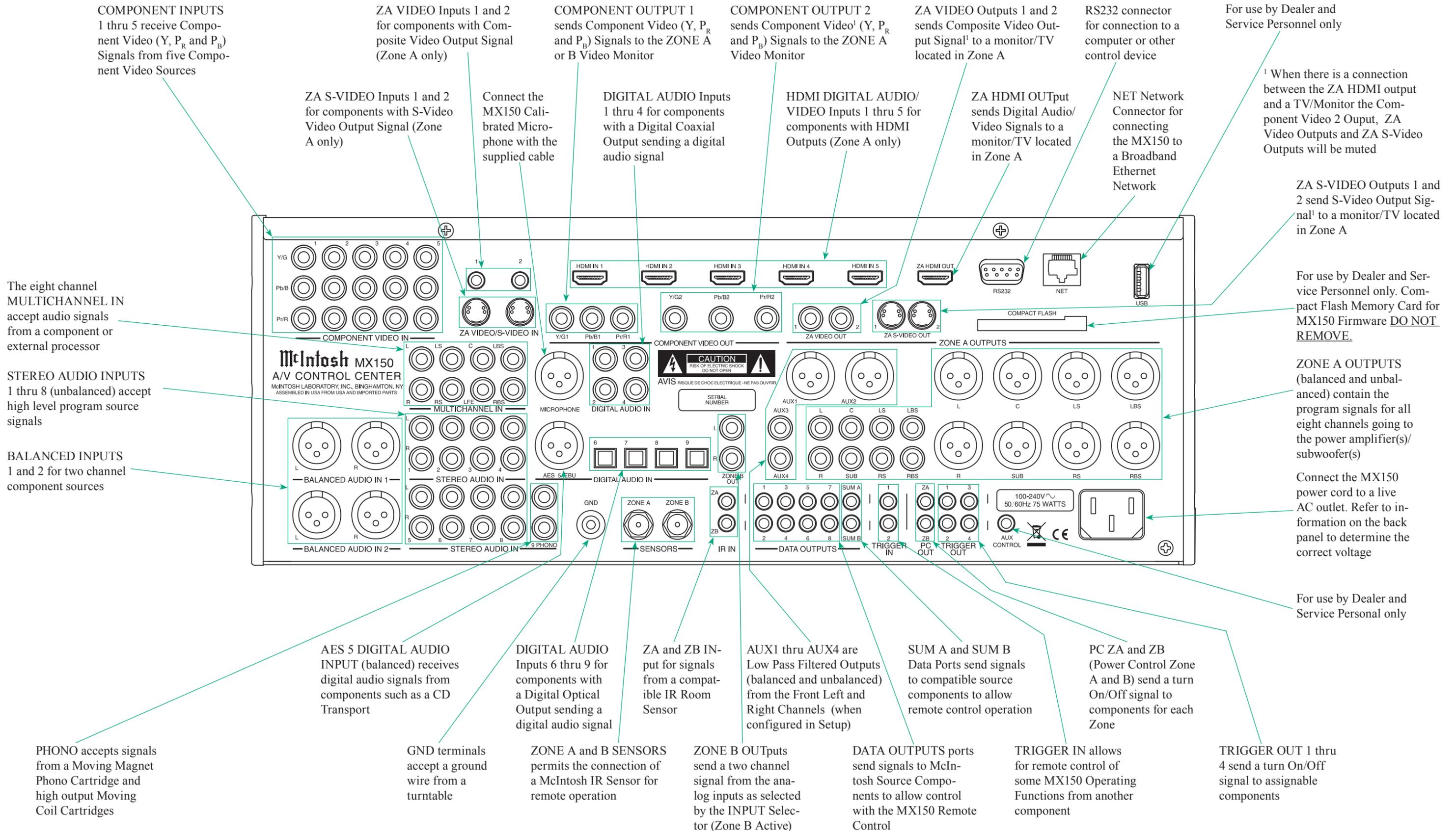
INPUT Control allows the selection of various sources for listening and viewing in Zone A and Zone B
