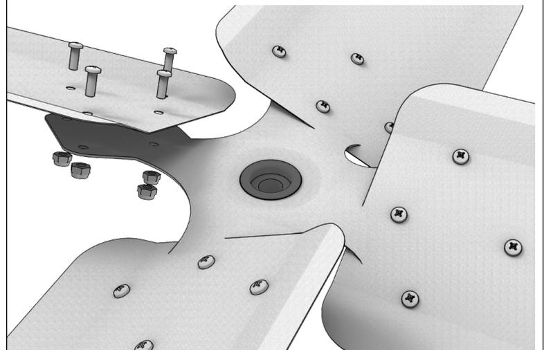
Example of 4-blade unit with hub facing toward motor
