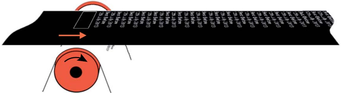
The next print is performed when the ribbon speed is the same as the substrate speed.
