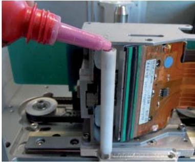
Fit a new Peel roller body over the shaft and secure the screw with Loctite 222.
