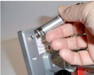
Place the damaged roller to the side.
