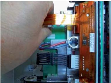
Remove the ribbon connector from the printer interface PCB.
