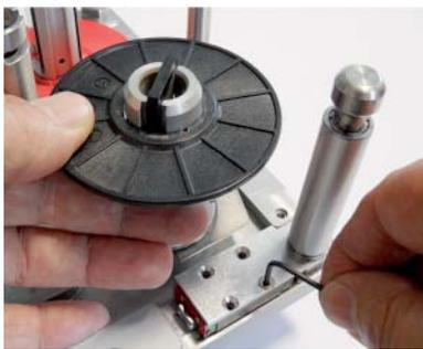
Secure the screws with Loctite 222.
