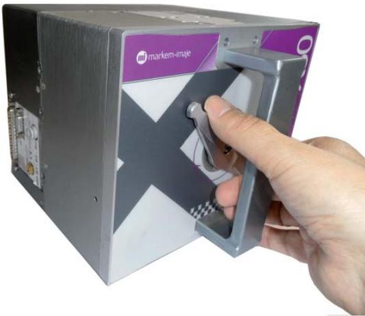
1 Rotate the locking lever on the cassette to the OPEN position.
