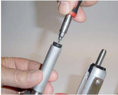
Remove the securing screw on the end of the roller.
