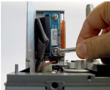
Remove the two retaining screws from the ribbon connector block.
