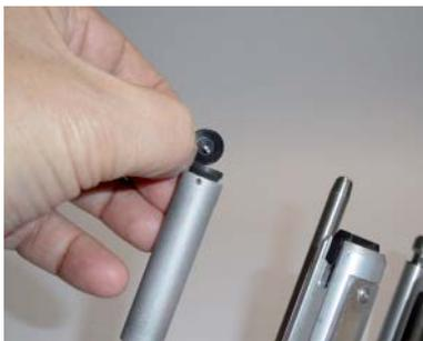
Remove the screw and securing washer.
