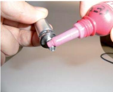
Before fitting a replacement roller, apply Loctite to the screw thread at the base of the roller.
