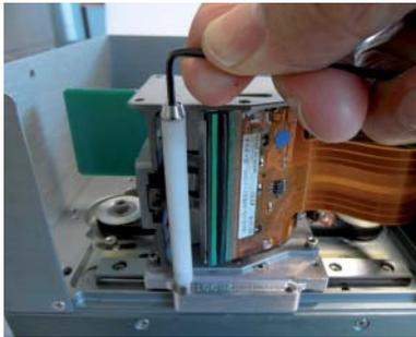
Remove the retaining screw from the end of Peel roller.
