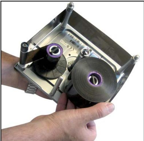
Pull the ribbon forward using the ribbon take up reel flange located below the ribbon.
