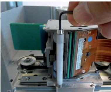
Once the seal has been broken at the base of the screw, use an Allen key to unscrew the Peel roller.
