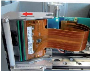
Move the print module to the side to allow access to the ribbon cable connector.
