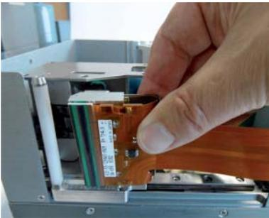
Remove the printhead from the print module.
