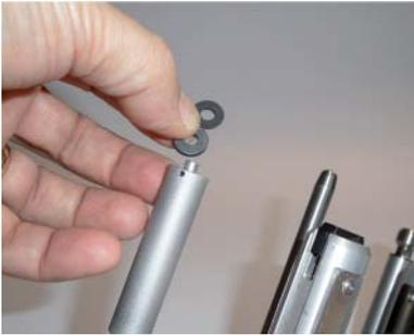
Remove the damaged magnet and rubber washer.
