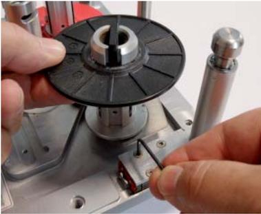
Remove the four retaining screws from the tension roller carriage.
