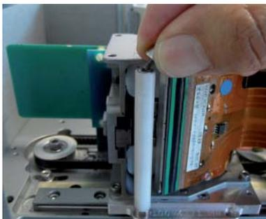
Remove the screw and washer.
