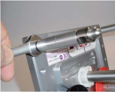
Remove the damaged roller by applying a spanner to the two flat surfaces at the base of the roller.
