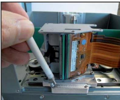
Remove the roller from the printer carriage plate.
