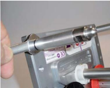
Ensure that the Roller is free to rotate.
