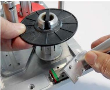
Remove the damaged tension roller assembly.
