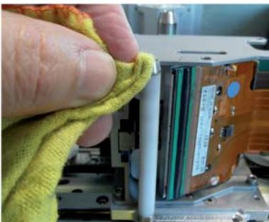
Clean off any excess fluid and ensure the roller is free to rotate.
