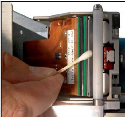
Use a cotton swab or a soft cloth soaked in Isopropanol solvent to remove any residue from the printhead. Take care not to use excessive amounts of solvent.
