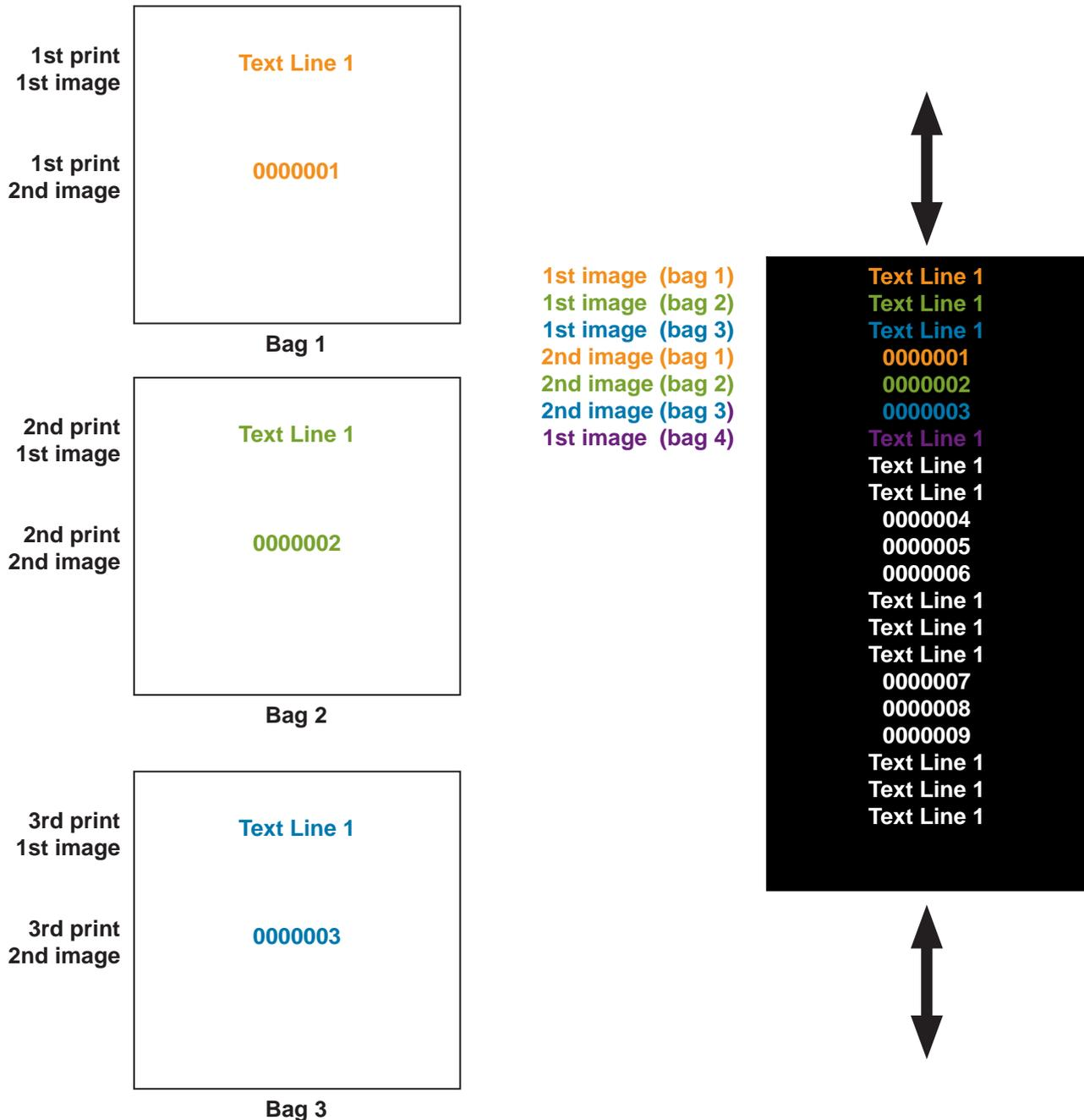
The ribbon is shuttled backwards and forwards until all of the available unused ribbon is utilised. The printer will then start the printing sequence again with bag 4.
