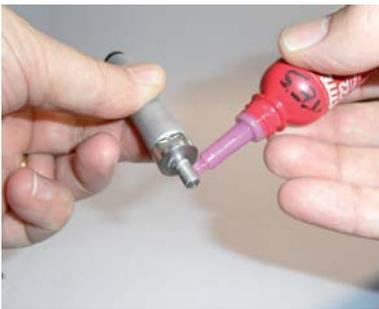
Before fitting a replacement roller, apply Loctite 222 to the screw thread at the base of the roller.
