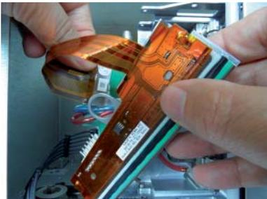
Remove the printhead from the print module.
