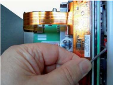
Remove the retaining screw from the printhead
