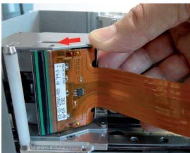
Push the printhead forward towards the peel roller and rotate the rear of the printhead outwards as shown above.
