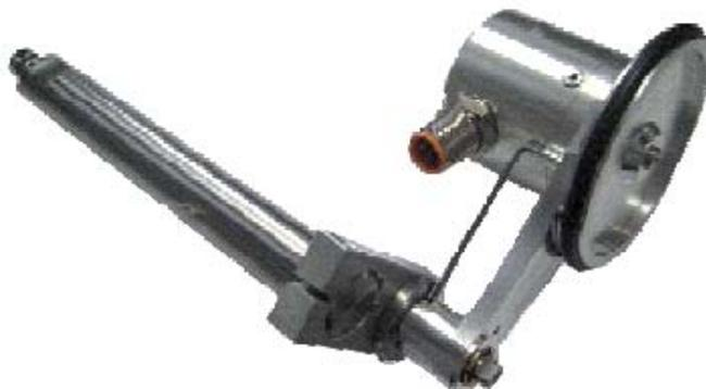
A high resolution encoder (6122 pulses/rev) should be used where print speeds lower than 70mm/s are experienced during the print cycle. This is also the case if the packaging machine exhibits high acceleration from low speeds.
