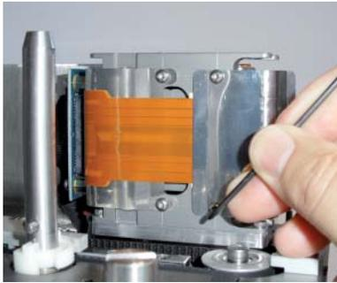
Remove the retaining screws from the printhead ribbon cable guide.
