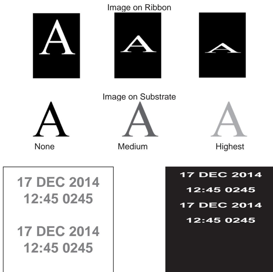
**Note:** In situations where the substrate runs very slowly it is possible for the ribbon to run faster than the substrate in order to achieve a print.
