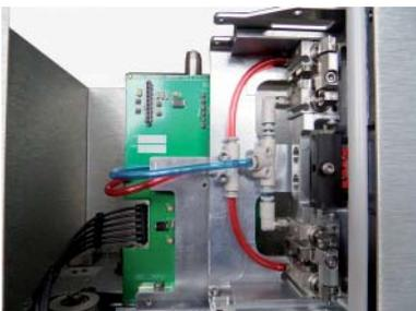
Remove the printhead from the printer body.
