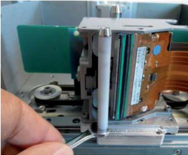
If the peel roller shaft has been damaged, undo the retaining nut at the base and remove the complete assembly.
