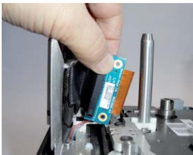
Disconnect the ribbon cable from the PCB.
