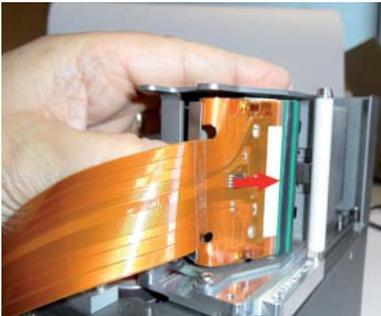
Push the printhead forward towards the peel roller and rotate the rear of the printhead outwards as shown here.
