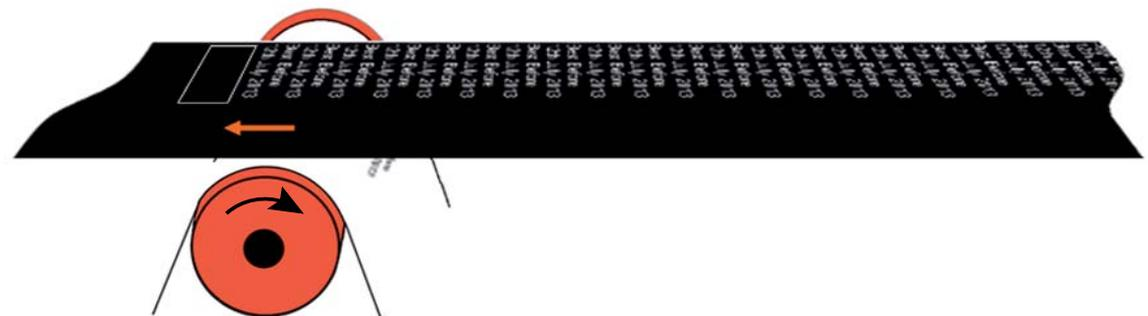
Matching the 'Max substrate speed' to the actual maximum substrate speed will allow the SmartDate X60 to run at the highest pack rate possible.
