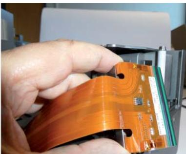
Remove the printhead from the print module.
