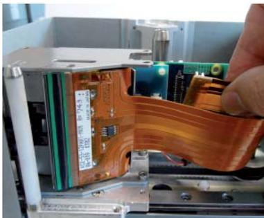
Disconnect the ribbon cable from the printer interconnection PCB.
