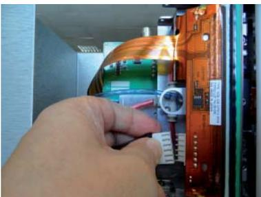
Remove the power connector from the Printhead.
