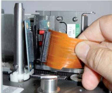
Remove the ribbon cable from the connector.
