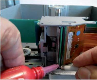
Fit a new peel roller assembly and ensure that it is secure and free to rotate. Secure with Loctite 222.
