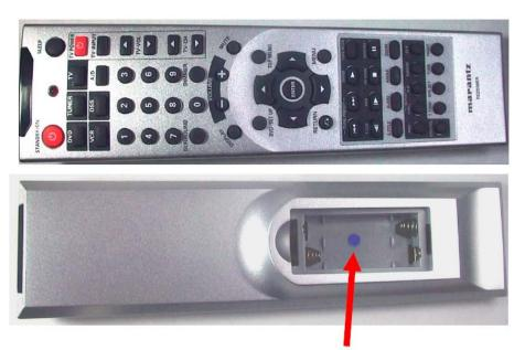
As for improvement the remote controller, the blue label is stuck on the Battery compartment.
