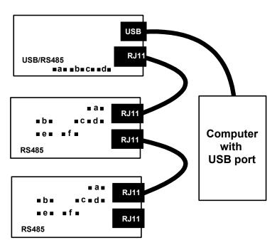
meter. The RJ11 output of each RS485 meter can then be connected to the next meter via a 6-conductor straight-through data cable. Up to 30 additional meters may be daisy chained and be addressed using the Custom ASCII Protocol.
