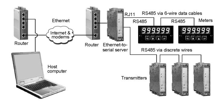
With an Ethernet connection, our Nodes and the host PC can be connected directly to the same LAN, and our software will automatically discover all our Nodes in the LAN. A Node cannot be connected directly to a PC via an Ethernet cable.
