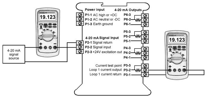
Method 2. Place identical resistors in the input and output legs and measure the difference of the V = IR voltage drops across the two resistors. Adjust the S potentiometer until the meter reads zero, which indicates that the input and output currents are the same.
