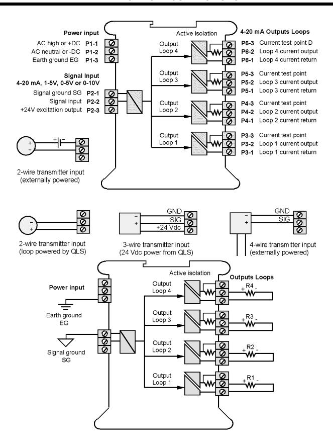
**Floating loads:** Any output load R that is floating (not connected to a local ground or earth ground) can be connected between current output (Pin 1) and current return (Pin 2). Current return is internally tied to signal ground SG, which can be floating or be connected to earth ground. Loads have to be passive (or sinking).
