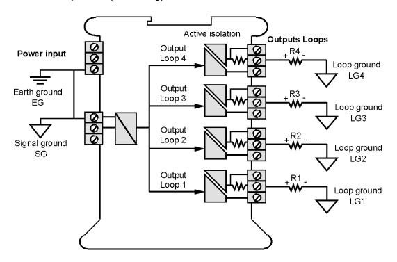
**Grounded loads:** Any output load R can be connected to a local loop ground LG instead of current return. The loop grounds LG can each be different, but can only differ from signal ground SG by a common mode voltage CMV, which is defined as  $V_{LG}$  -  $V_{SG}$ . Signal ground SG must be tied to earth ground EG or be within 1 Volt of EG.
