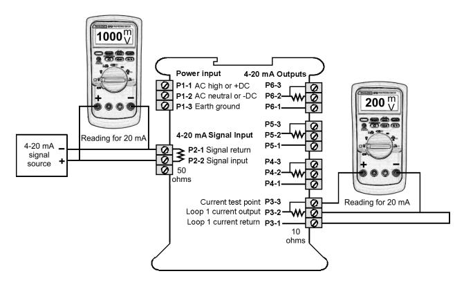
On the input side, the resistance across the P2-1 current input and P2-1 current return terminals is 50 ohms  $\pm$  0.25%. With a 4-20 mA signal, the measured V = IR voltage drop will be 200-1000 mV.
