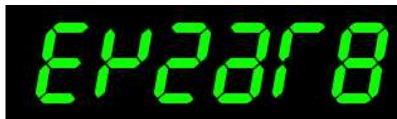
Example of Mirror Reverse display displaying the number 876543
