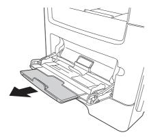
Fully pull out the extension guide of the Manual Feed Tray.
