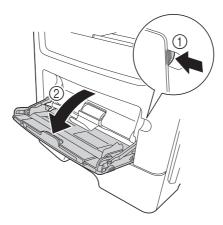
2 Pull out the extension guide of the **Manual Feed Tray**.
