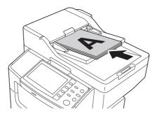
→ Load the original so that its top side is placed at the back. When loading in a different orientation, be sure to specify the loading direction of originals.
