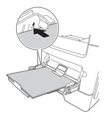
→ For letterhead, load paper first from the top edge with the letterhead side facing up. For 2-sided printing, load paper first from the bottom edge with the letterhead side facing down.
