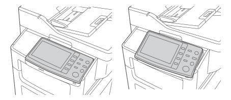
To adjust the angle of the Control Panel, tilt the Control Panel up and down.
