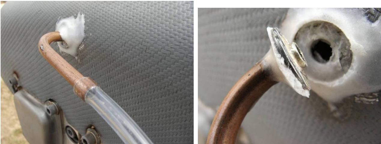
Figure 61: Ram Air duct pressure tapping.
