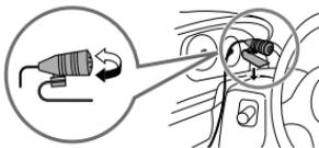
Secure using cord clamps (not supplied) if necessary.
