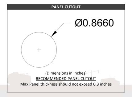
Note: If using switch as part of the Intellitec kit number 10-01118-000 refer to the dimensions above for mounting the switch in the wall.
