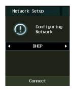
IP, Net mask, Gateway and DNS should be entered in case of using manual IP in network setup.
