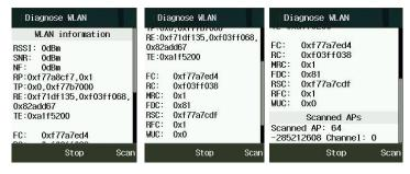
The diagnosis of wireless communication surroundings is possible to find out the connection from ICW-1000G to AP, the units of AP around and inside of the present-connected channel, and variables of the surroundings through diagnosing the status of wireless local area
