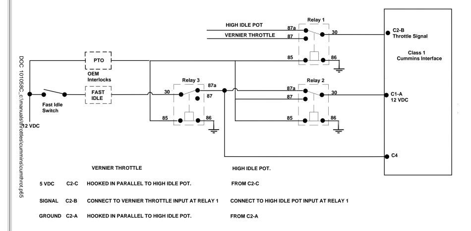
RELAY 3 DISABLES HIGH IDLE WHEN OK TO PUMP/PTO ENGAGED SIGNAL IS PRESENT
