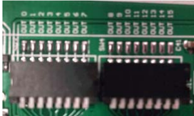
Figure 2. Output polarity selection switches.
