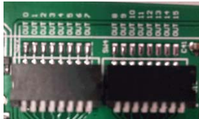
Figure 1. Output polarity selection switches.
