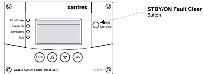
**Figure 15** Xanbus SCP **STBY/ON Fault Clear** Button
