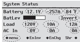
**Figure 17** Bulk System Screen (Example)
